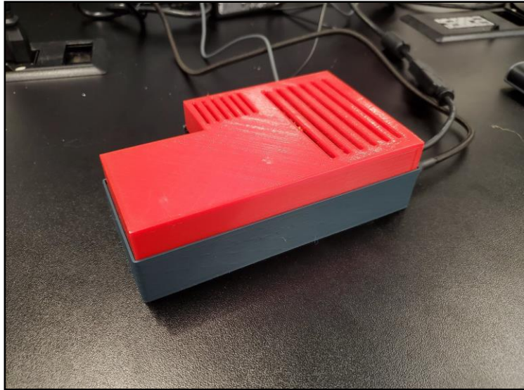
Figure 9: Computational Prototype Housing 3D Printed Assembly
